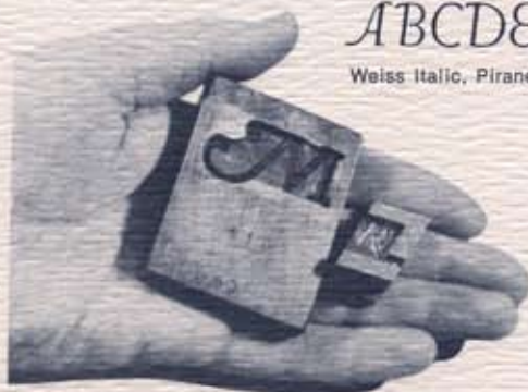
Matrix for 60 point Bookman swash M (ATF), and 36 point Ludlow Caslon Italic swash R.
